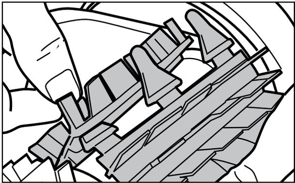
**Figure 17. Pull Tabs Through Each Slot**
