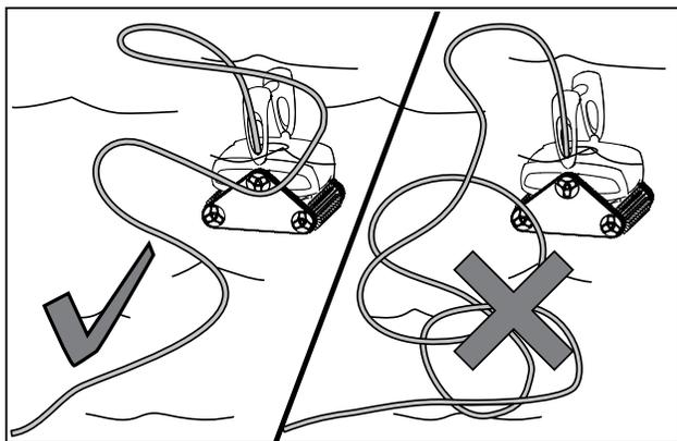
Figure 12. Correct Floating Cable
