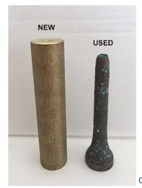
The mineral electrode is sacrificial and designed to slowly disintegrate. After an average of 12 months, depending on conditions, the electrode will wear away and require replacement. You will know this when it is 'pencil thin', or about 1/4 inch at the centre.
